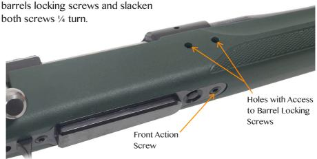
Using the same wrench, slacken the front action screw in front of the magazine ¼ turn. The barrel can now be slid forward into the barrel channel and lifted clear. When re-fitting insert the barrel with the notch facing down. Rotate whilst pulling back gently until the notch engages and the barrel goes fully home.
