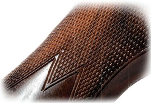
The chequering is not laser cut as this produces vertical sided diamonds that break off easily. The Schultz & Larsen chequering is cut with a 45-degree cutter to provide perfect pyramids, the strongest and hardest wearing chequer pattern.
