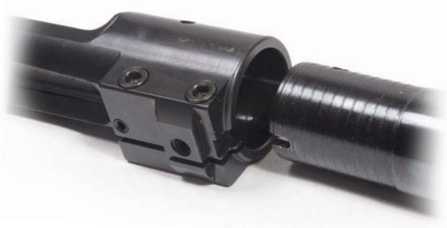
Safety has top priority with all locking parts designed and tested to withstand at least three times normal load. In the case of an overload resulting in a primer blow-out or case rupture, the high pressure gas can escape through holes in the front of the action and on the side of the bolt. This, coupled with the extremely tight fit of the bolt and action, ensures that the shooter is not injured.
