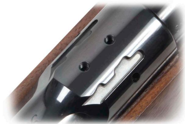
The top of the action accepts the strong and lightweight Schultz & Larsen all steel scope mounts, available in a range of diameters and heights. The action is drilled and tapped for those who wish to use an alternative mount (hole spacing is 12.5mm and action radius 15mm).
